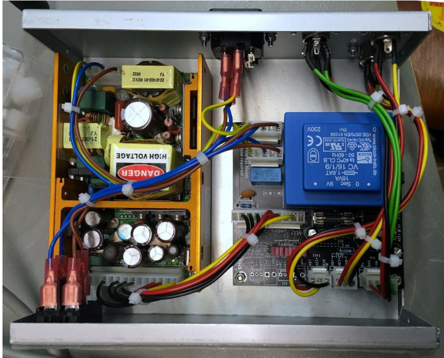
Figure 27: Finished PSU in TEK0 384 case
